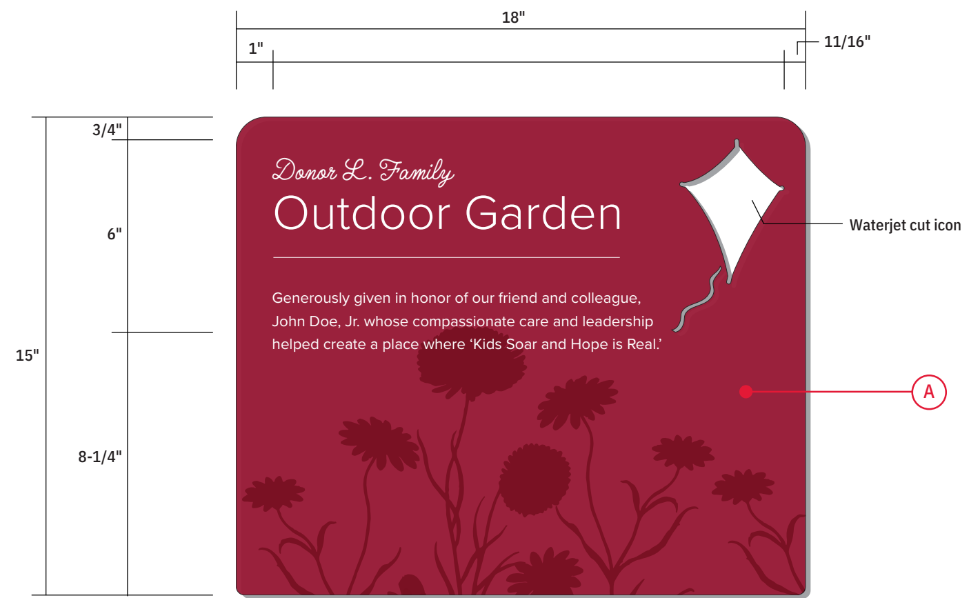
1 DN-09 Exterior Donor Sign Front Elevation Scale: 3" = 1'-0"
